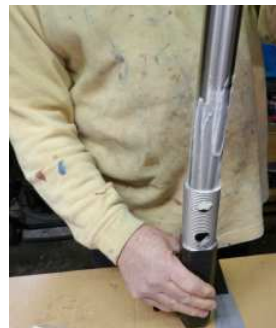
Stainless Steel Glass Brackets & Stainless Steel Post that Epox-E-Glue applied & Slid were a sloppy good Fit
