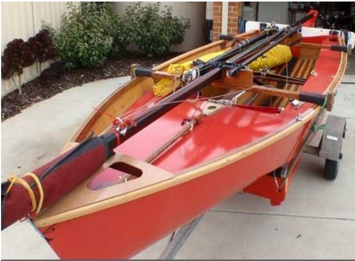
Figure 3 - Rolled finish using Aquacote water based polyurethane marine paint
