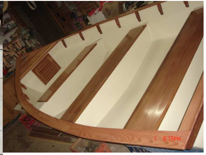
Figure 4 – Dolphin 12 built using Bote Cote & finished using Aquacote
