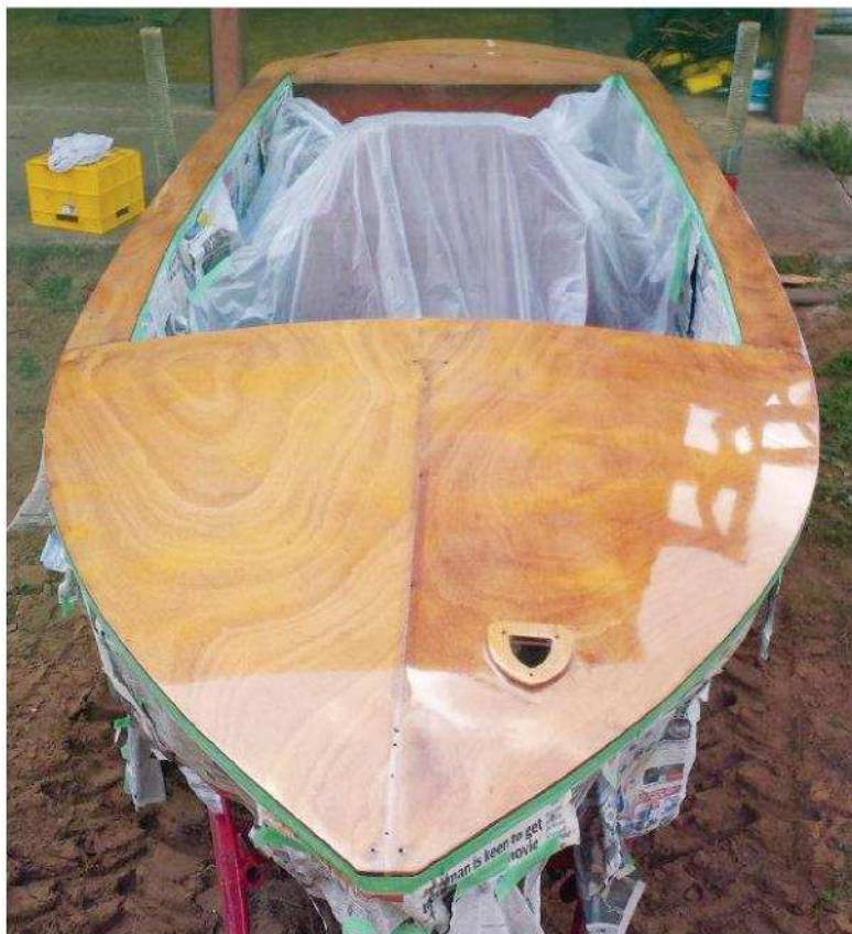
Mate you are a legend – four wet coats with 50% water applied with a wet rag ... nailed it. Thanks for your help!
