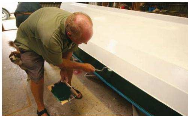
Armfield's Slip, kit St Ayles Skiff sheer plank. Incidentally this can had been partly used, then sat on my shelf for about 10 years! Worked a treat. Note: Andrew is using the scrap ply palette to load his Unipro Mohair blend HDHD75 roller sleeve, which you can find in Bunnings OR much cheaper from BoatCraft Pacific agents around Australia. This is also by far the best epoxy resin roller sleeve I've ever used. Doesn't seem to break down even with prolonged use. May be washed out with white vinegar if using epoxy resin.
