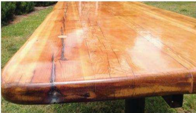
AquaCote Varnish applied 50:50 – clean water and rag, SA.
