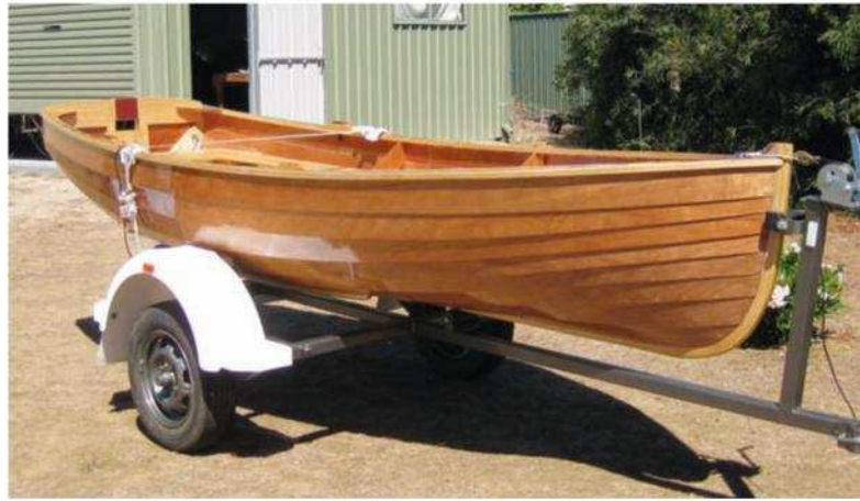
Alan Carson used a hair brush to apply his AquaCote Clear over Bote-Cote on his concours kit Guillemot. Note the reflection near the mudguard!
