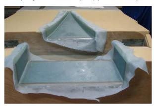
Figure 3 -Peelply applied to Cosy Aircraft components
