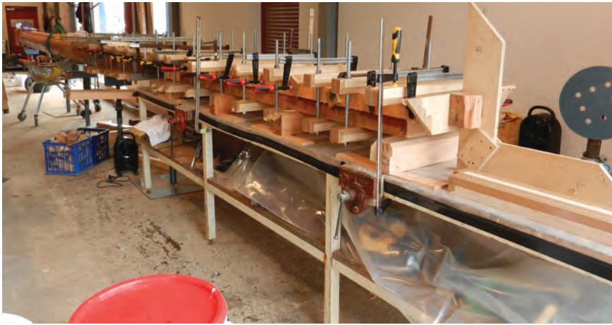
Figure 3 – First side glued and clamped.
