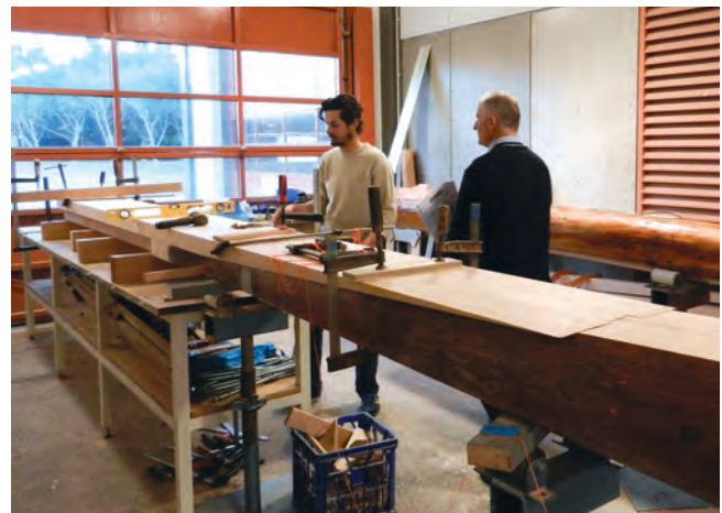
Figure 2 – Chamfered section of mast.
