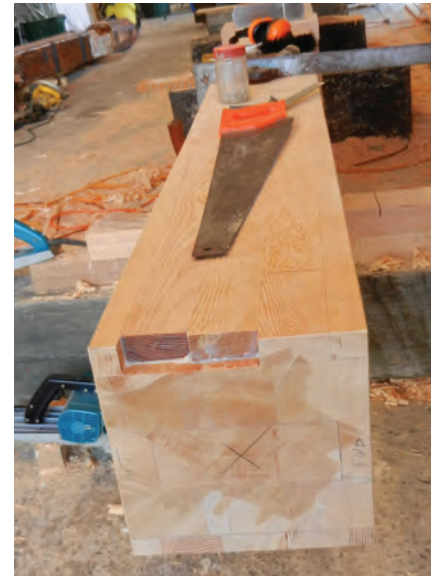
Figure 4 – Square section at completion of glueing.
