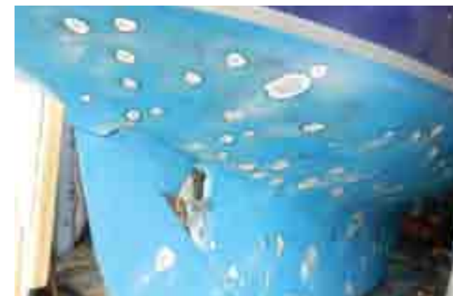
Figure one – Osmosis damage ground out.
