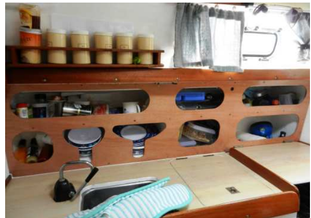
Figure 4 – New 3mm Gaboon Ply Stowage sealed with Clear System
