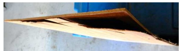
Figure 2 – 4mm Tropical Hardwood Delamination
